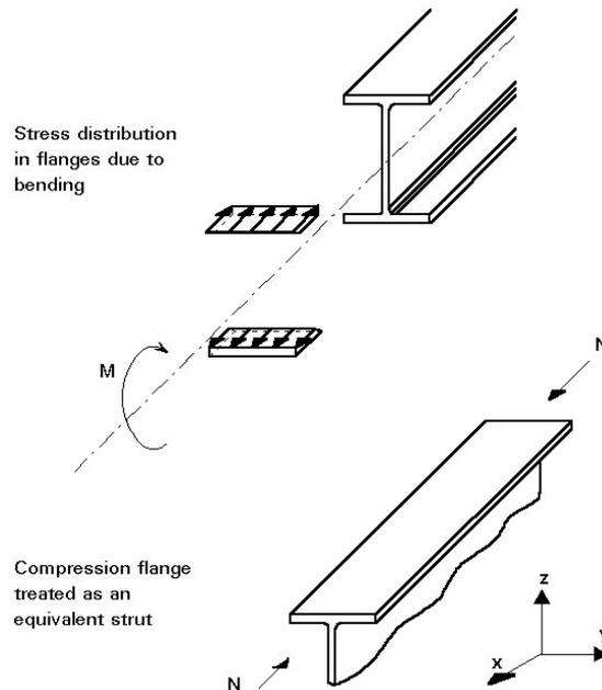
Figure 11 – Approximation of beam buckling problem as a strut problem.
