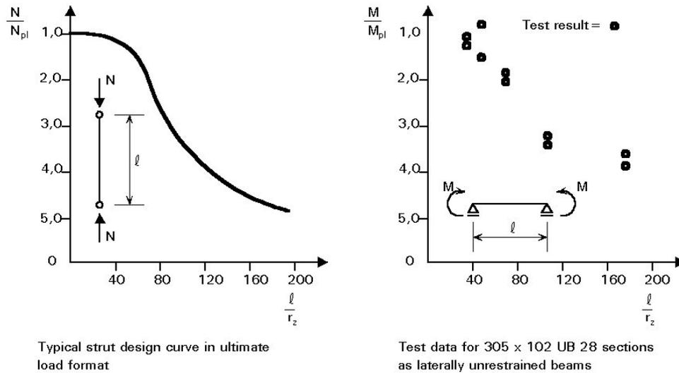
Figure 4 – Dependence of the beam strength on unrestrained length and analogy with column strength.
