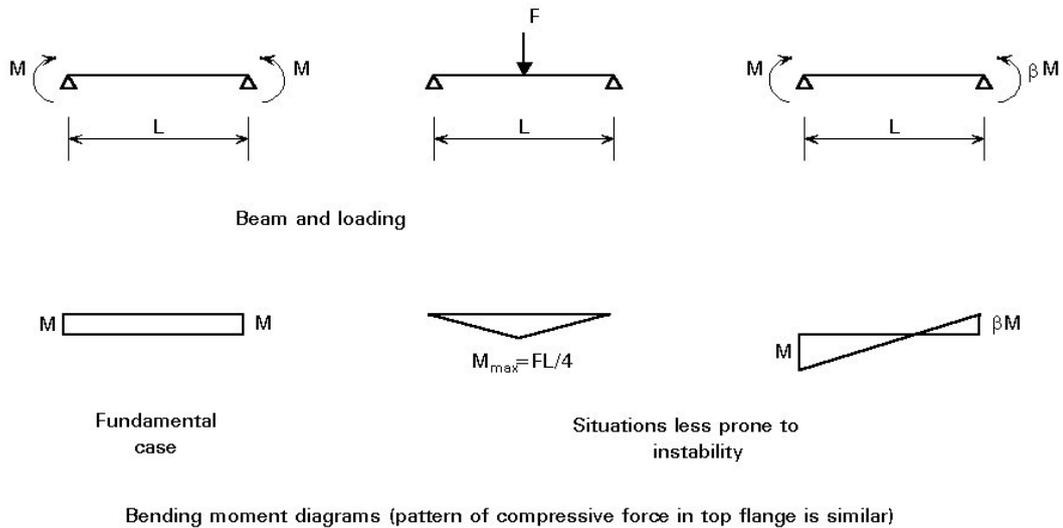
Figure 12 – effect of non-uniform moment on lateral –torsional buckling.
