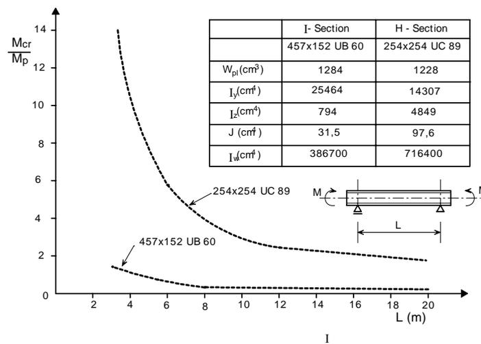
Figure 10 - Comparison of elastic critical moments for I and H sections.
