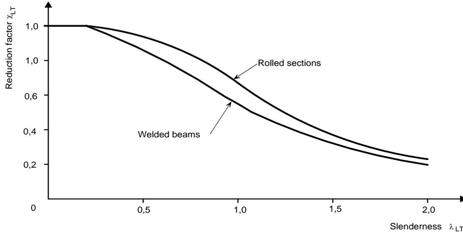
Figure 18 Lateral-torsional buckling reduction factor
