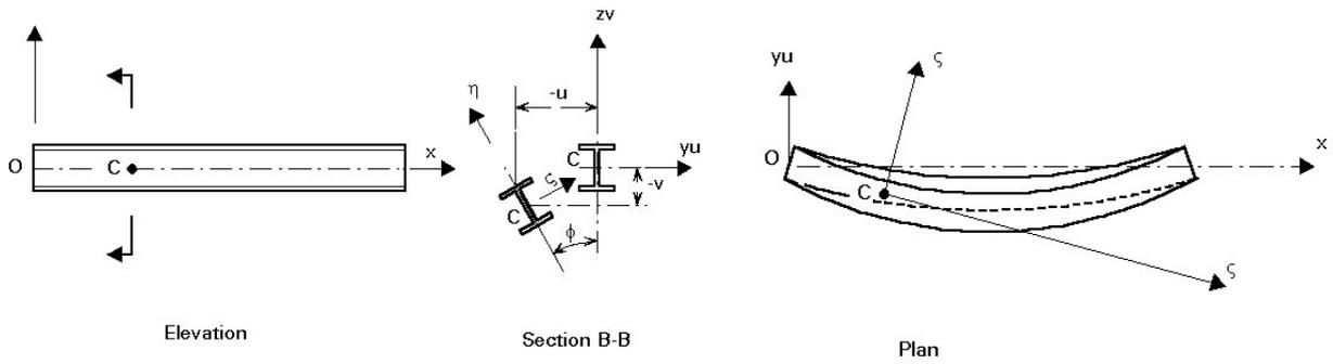
Figure 6 – Deformation of a beam.
