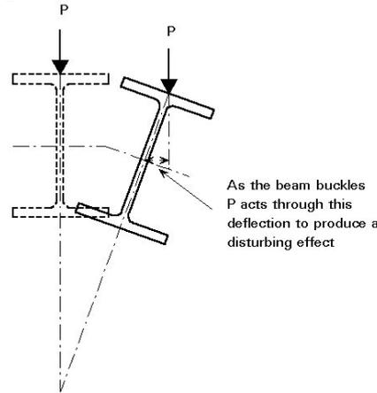
Figure 22 – Destabilising loading.
