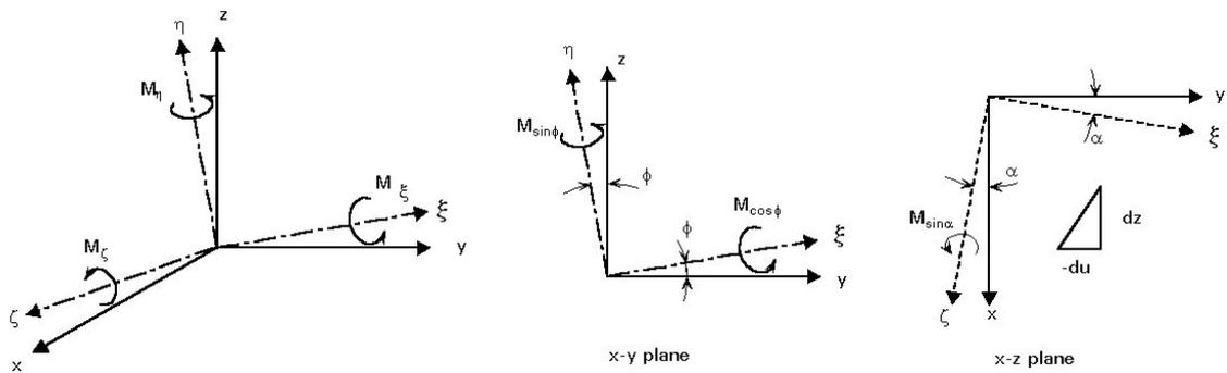
Figure 8 – Resolution of applied end moment  $M$  into components about the deformed axes.
