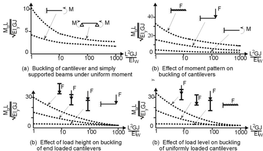
Figure 24 – Buckling of cantilever beams.
