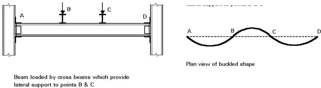
Figure 14 – Buckling of beams provided with lateral bracing.
