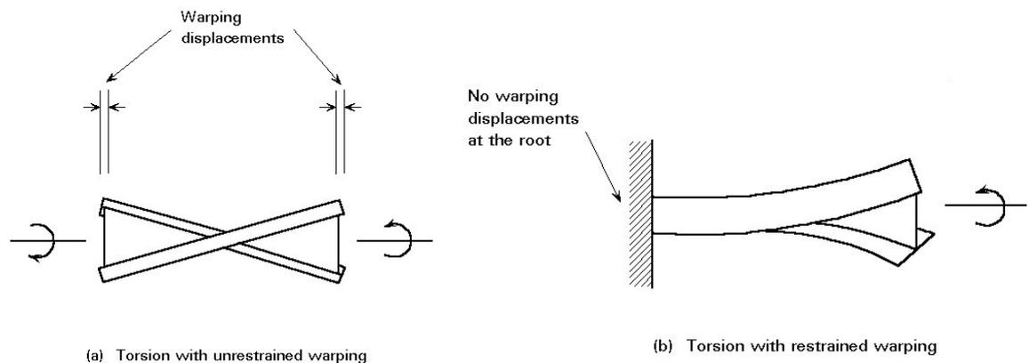
Figure 7 – Torsion boundary conditions.
