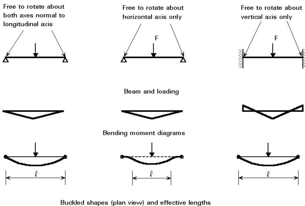
Figure 13 – Effect of restraint in plane or elevation on lateral –torsional buckling.
