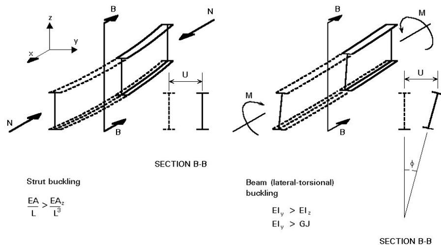
Figure 3 – Similarity between strut buckling and beam buckling.
