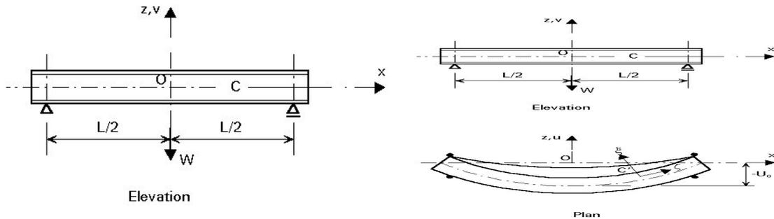
Figure 26 – Buckling of a beam with a central transverse load.
