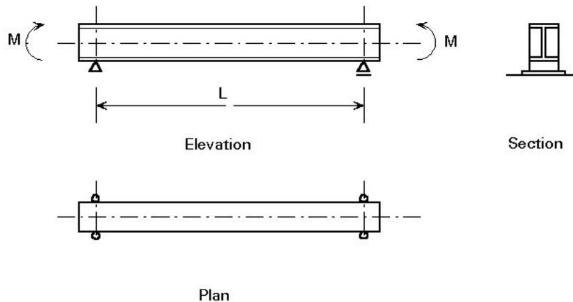
Figure 19 - Definition of basic lateral-torsional buckling problem.
