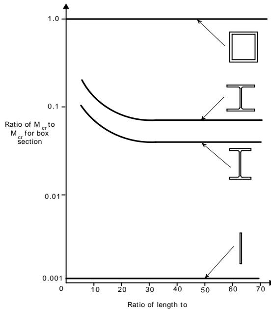
Figure 9 - Effect of cross section shape on theoretical elastic critical moment.
