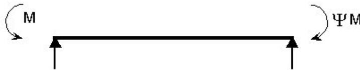
Figure 21 – Moment gradient loading over beam span  $L$ .
