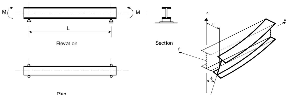
Figure 5 - Lateral torsional buckling of a simple I beam under uniform moment.
