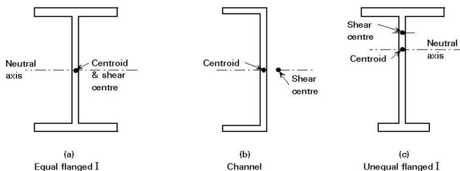
Figure 17- - Equal flanged section and examples of sections with one axis of symmetry.
