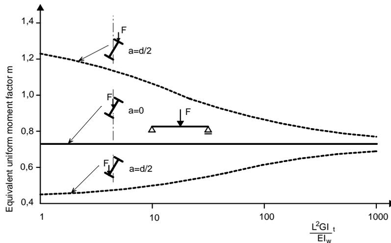
Figure 23 - Effect of level of load application on beam stability
