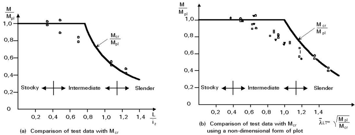
Figure 16 - Comparison of test data with theoretical elastic critical moments
