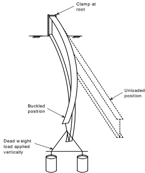
Figure 2 - Lateral-torsional buckling of a slender cantilever beam.
