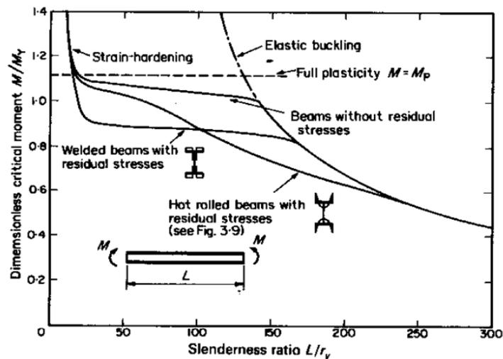
Figure 15 - Lateral buckling strengths of simply supported I beams.
