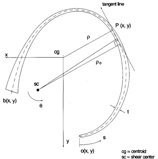
Note: All directions are shown positive;  $\rho$  and  $\rho_o$  are positive if they are on the left side of an observer at  $P(x, y)$  facing the positive direction of  $s$ .
