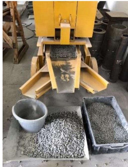
Figure 3 View of the crushed concrete to make the RAC
