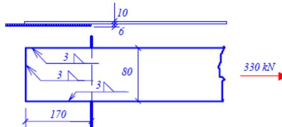
The structural welds should be (i) longer than  $40 \text{ mm}$ , and (ii) longer than  $6 a_w = 6 * 3 = 18 \text{ mm}$ . Both of these are satisfied. The full length of the weld can be taken into account in the strength calculation, because  $150 a_w = 50 * 3 = 450 \text{ mm} > 170 \text{ mm}$ .
