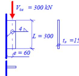
The structural welds should be (i) longer than  $40 \text{ mm}$ , and (ii) longer than  $\delta a_w = 6 * 4 = 24 \text{ mm}$ . Both of these are satisfied. The full length of the weld can be taken into account in the strength calculation, because  $150a_w = 50 * 4 = 600 \text{ mm} > 300 \text{ mm}$ .
