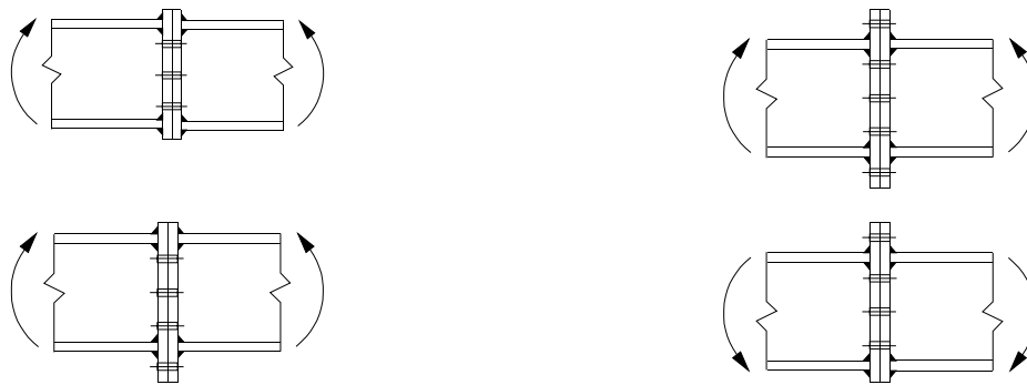
Figure 6.18: Bolted beam splices with welded end-plates
