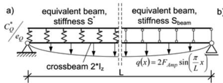
Figure 4: strut models, a) for calculation of  $S^*$ , b) for determination of  $S_{beam}$
