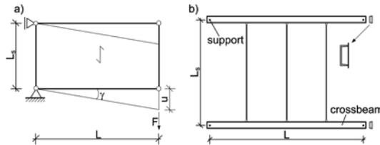
Figure 3: Test setup, a) : shear panel construction, stressed by shear, at 4 edges connected to substructure, b) beam construction, stressed by transverse forces, at 2 edges connected to substructure
