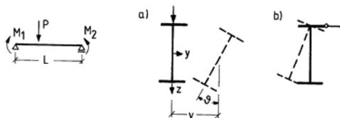
Figure 1: Lateral torsional buckling of beams: a) laterally unsupported, b) laterally supported
