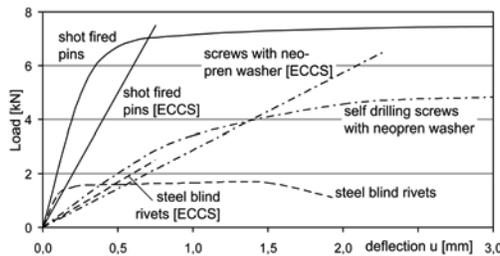
Figure 2: Example for load-deflection curves for different kinds of fasteners, a thickness of sheeting  $t_N = 0.75$  mm and a profile 39/183 mm [8]
