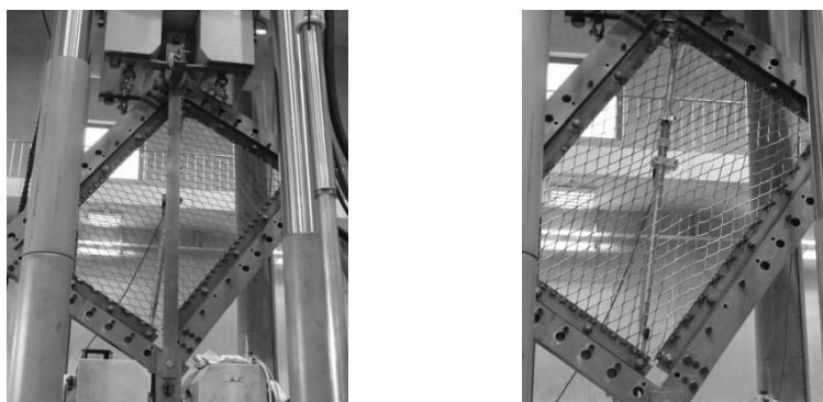
Figure 5 – Two possibilities of erecting EMP to the testing frames (left: sens1; right: sens2)
