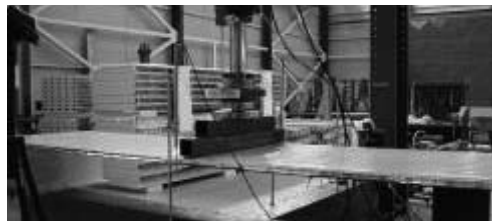
Figure 10: Experimental set-up of the test on of a single span panel subject to a line load.
