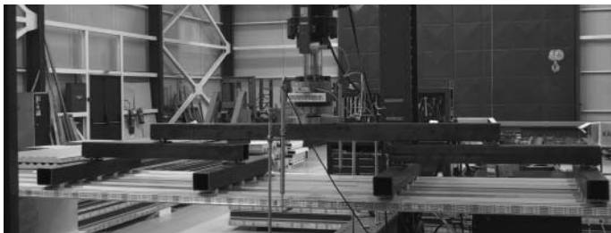
Figure 7: Experimental set-up of the four-point bending tests.
