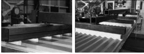
Figure 8: Timber loading platens on the trapezoidal profiled face (left) and special cuts of the panels on the waved profiled face (right).
