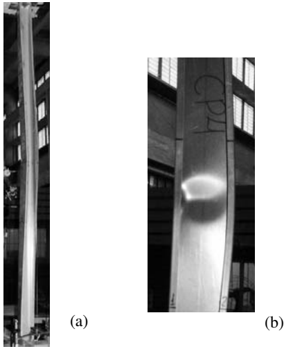
Figure 4: Column (a) flexural-torsional deformed configuration and (b) local collapse mechanism.
