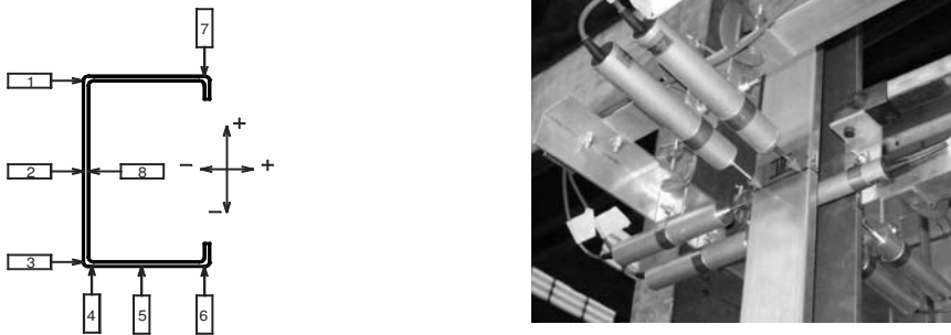
Figure 3: (a) Position of the displacement transducers around the column cross-section and displacement sign convention, and (b) view of the displacement transducer positioning at the column mid-height.
