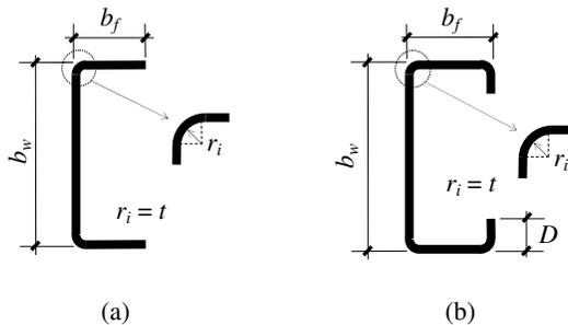
Figure 1: Cross-section of columns to be optimized: a) C-section without lips; b) C-section with lips
