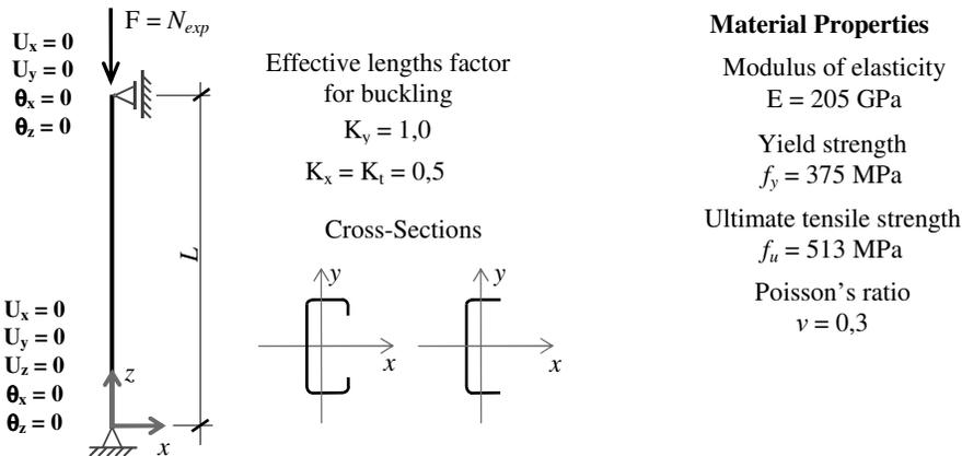
Figure 2: Reference system and boundary conditions of the columns optimized
