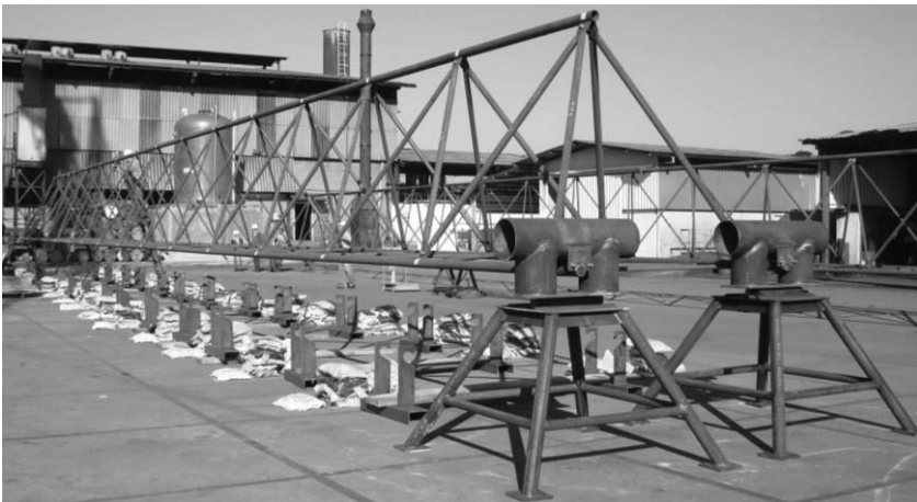
Figure 6: Truss prepared to begin the experimental analysis.
