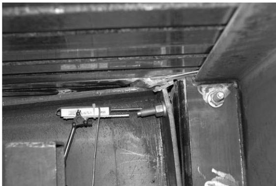
Figure 12: Severe buckle at column face and end plate.
