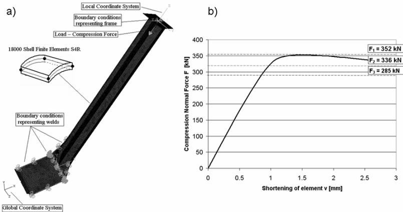
Figure 10: Compression bar: sub-model (a) and statical path of equilibrium of compression member (b)
