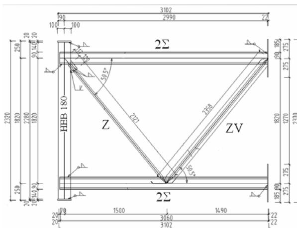
Figure 2: Geometry of truss made from cold-formed sections.
