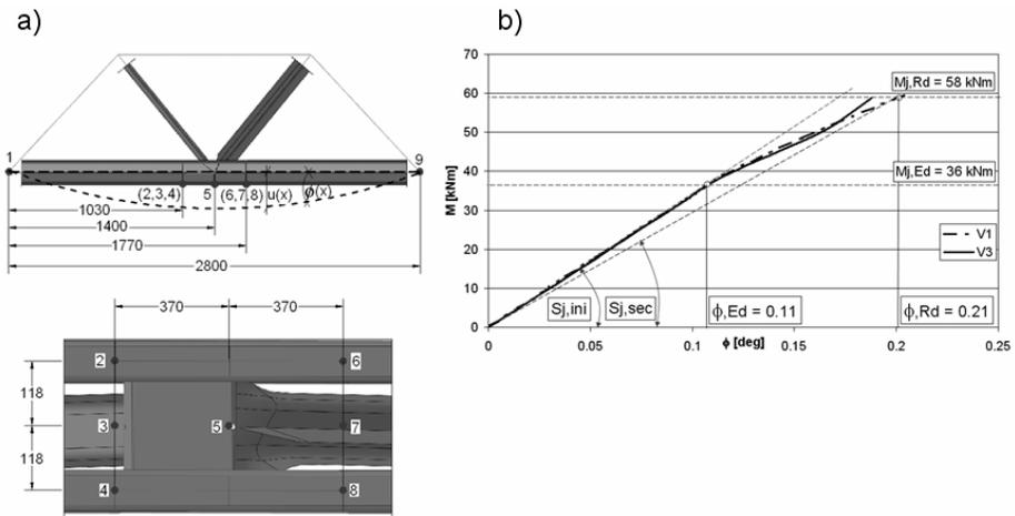
Figure 7: Measurement points for displacements (a), bending moment-rotation curve (b)
