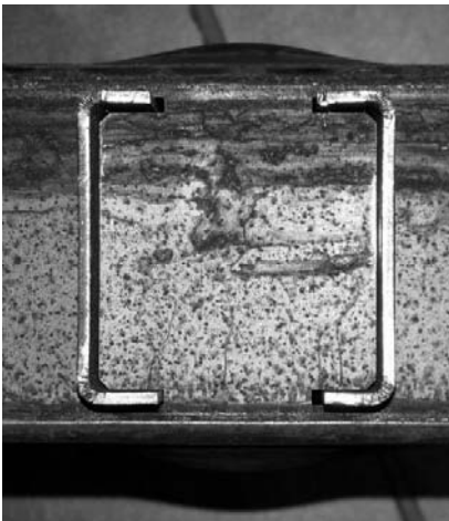
Figure 9: View of chord webs failure WTL3 Figure 10: View of chord face and webs failure WTL3
