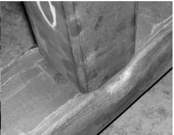
Figure 9: View of chord webs failure WTL3 Figure 10: View of chord face and webs failure WTL3
