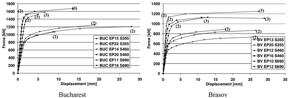
Figure 6: T-stub behavior according to numerical analysis
