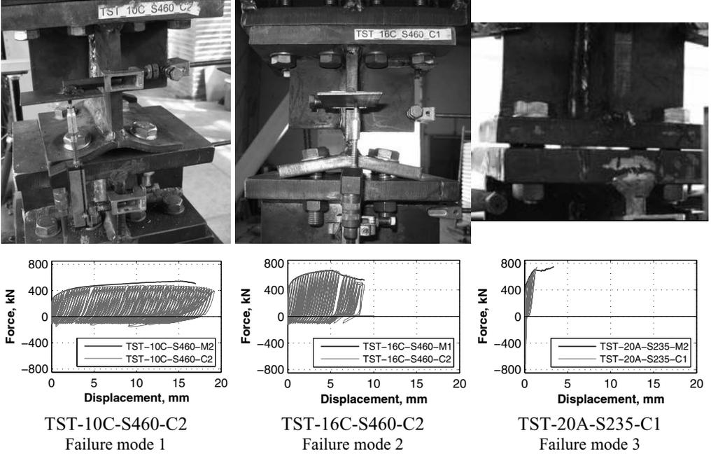
Figure 1: Examples of failure modes of T-stub specimens
