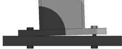
a) bolt-failure (specimen CCB1)
