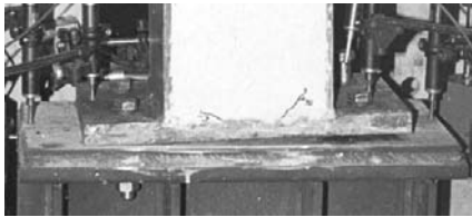
a) bolt-failure (specimen CCB1)
