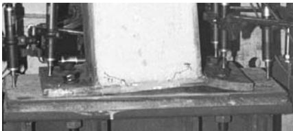
b) plate-failure (specimen CCB2)
