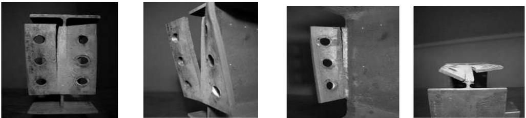
Figure 8: Partial depth endplate (test 4) failure mode.
