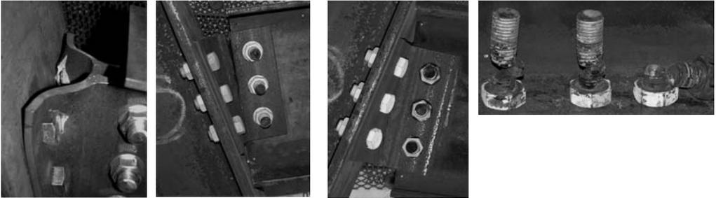
Figure 6: typical failure modes at 20°C, 450-500°C, and 650°C
