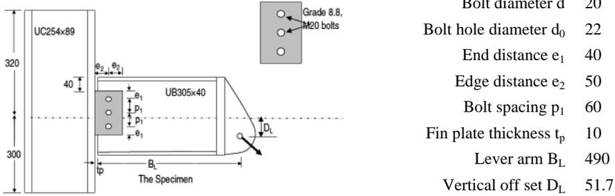
Figure 2: Fin plate test details.
