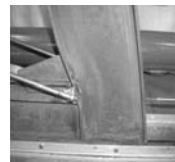
Figure 6: Details of WL 1320 column-beam-bracing joint deformations from tests and simulations.
