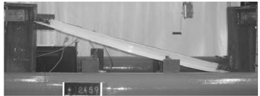
Figure 5: Frame deformation of bolted brace specimens from tests and numerical simulations.
