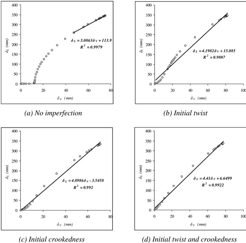
Figure 3: Plot of lateral displacement against vertical deflection
