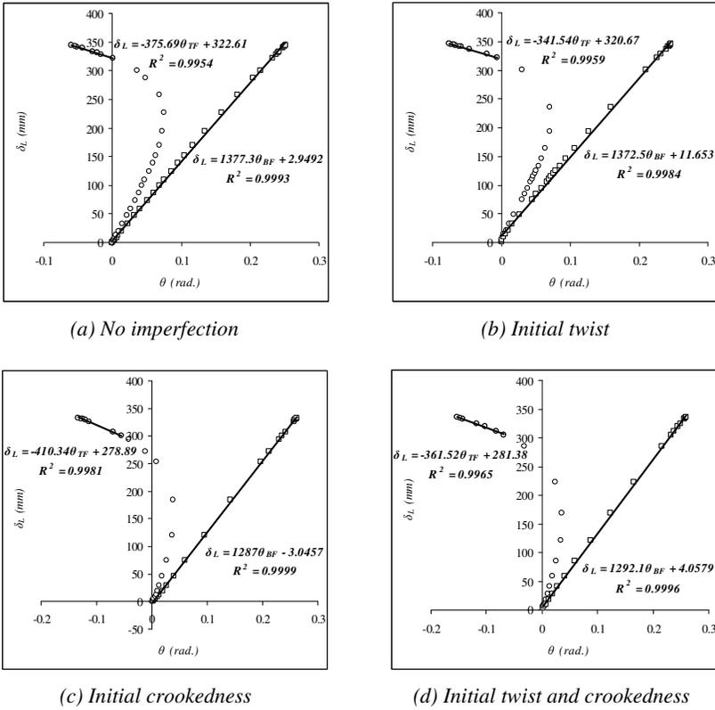
Figure 4: Plot of lateral displacement against angle of twist
