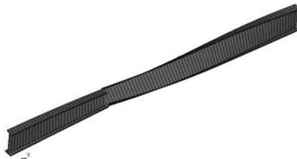
Figure 11: Lateral torsional buckling mode of tapered beam with moment hinge
