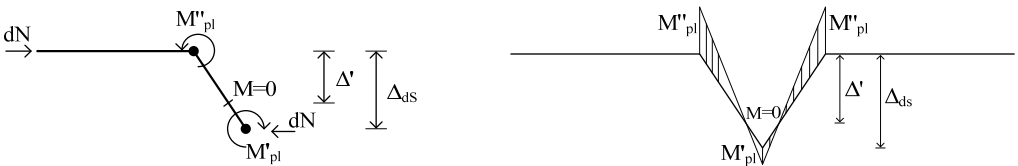
Figure 3. (a) Free body diagram and (b) bending moment diagram of the material strip.
